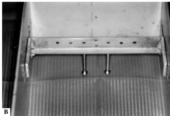
Figure 3 (A and B) Bottomless, lidless metal box (A) used to position rats to be radiographed. The box has two runners and two metal rods parallel to each other on the horizontal and sagittal planes (B).
